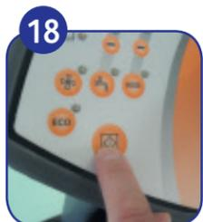
18 Press program start/stop button to deactivate all aggregates. It saves the last settings of several aggregates.
