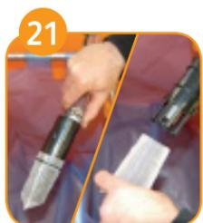
21 Remove filter sieve from water pump and clean under running water.
