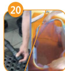
20 Drain recovery tank, then drain flexible solution tank, rinse recovery and solution tank with fresh water.
