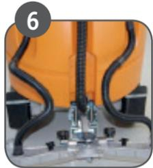
6 Mount suction hoses: bend hoses to the centre of the machine and plug these in the squeegee.
