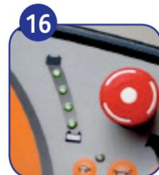
16 Green lights show battery level. If a red LED lights up, you have 10 minutes left to drive machine somewhere you can charge batteries.
