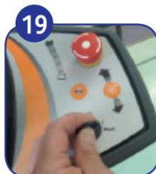
19 Turn the machine off by turning key anticlockwise.
