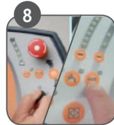
8 Turn the machine on by turning key clockwise. Press brush button for coupling tool(s) and press again to lift brush unit.
