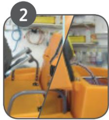
2 Lift seat to open tank cover for tank filling.
