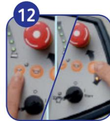
12 Press slow speed button to lower maximum driving speed. Press backwards button to change from driving forwards to backwards or vice versa.
