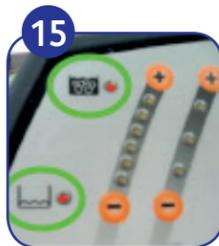
15 Red light indicates either full recovery tank (upper light) or empty solution tank (lower light). In both cases machine stops with normal sequence.
