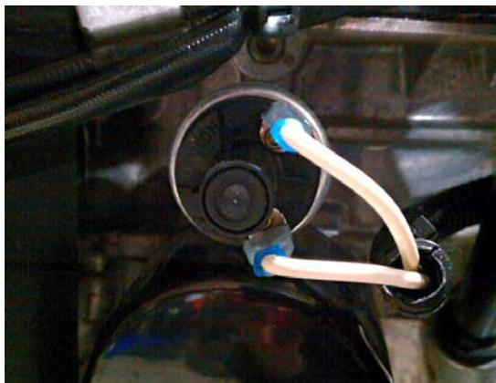
Locate the oil pressure switch just above the oil filter on the left side of the engine.
