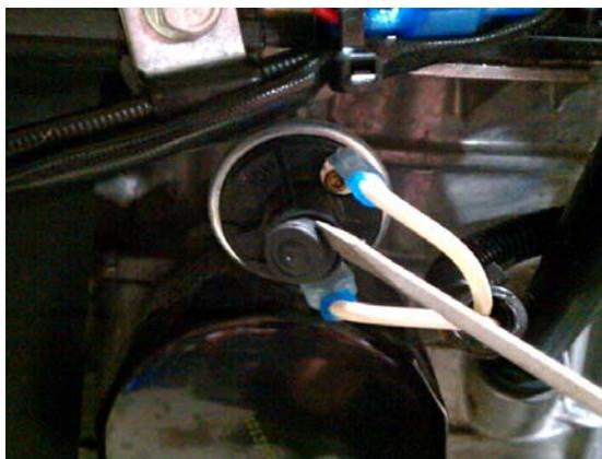
Remove the black, rubber seal on the end of the switch with a small screwdriver.
