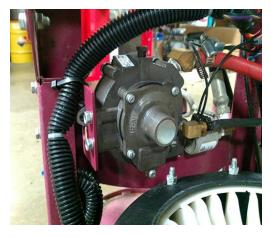
This picture is of a normal fuel regulator on a propane buffer.
