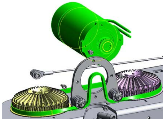
Picture 69: Brush belt & brush motor
