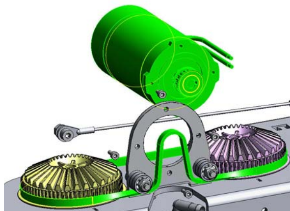
Picture 70: Brush belt & brush motor
