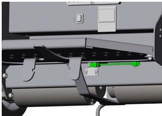
Picture 50: Limit switch
