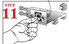
Adjust the temperature by removing the panel in front of the respective heater and turning the adjustment post. Wash temp. 155°F. Rinse temp.180°F.
