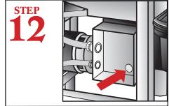
Remove the stainless steel plug to install the detergent probe (provided by your dispenser supplier; CMA does not supply).
