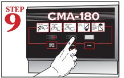
Press "AUTO FILL" immediately after power is turned on. Timer will automatically fill until the water overflows into the scrap trap. The initial fill may need to be pushed twice to fill wash tank.
