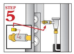
Remove the plug from the mixing chamber and install the rinse injection fitting (rinse injection fitting provided by your dispenser supplier; CMA does not supply).
