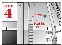
Remove the plastic plug to install the detergent fitting (provided by your dispenser supplier; CMA does not supply).
