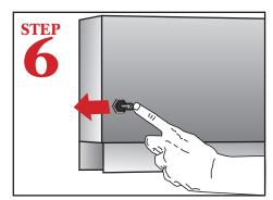
Push "RINSE TOGGLE SWITCH", located on the back of the control box, to fill the booster tank.
