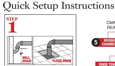
Connect a 2" drain pipe (not supplied) from scrap accumulator to floor or wall drain.
