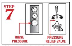
Adjust pressure regulator located next to cold water inlet, to 20 psi (maximum).
