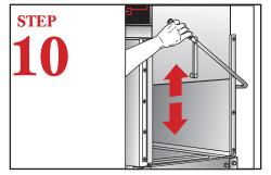
Open dishmachine doors completely. Closing the doors will automatically activate the machine.
