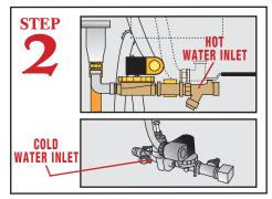
Connect dishmachine to hot water source 120°F -140°F. Connect cold water inlet (min 41°F and max 65°F). (Review other side for details).
