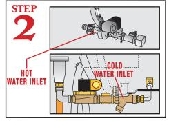
Connect dishmachine to hot water source 120°F -140°F. Connect cold water inlet (min 41°F and max 65°F).
