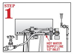
Connect Hot Water Supply Line to 1/2"Final Rinse Water Inlet. SEE STEP 11.
