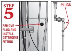
Remove plug to install detergent fitting. Remove plugs from the mixing chamber to install sani/rinse injection fitting (sanitizer, detergent and rinse injection fittings provided by dispenser manufacturer, CMA does not supply.)
