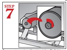
Remove motor cap to verify motor rotation. Shaft slot should be rotating clock-wise when motor is running. If shaft slot is turning counter clock wise, swap L-1 and L-3 on main contactor.
