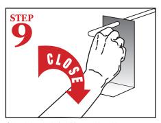
Close drain valve before filling machine with water.
