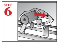
Remove the stainless steel plug to install the detergent probe (provided by dispenser manufacturer, CMA does not supply).
