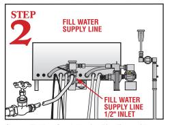
Connect Fill Water Supply Line (120F/140F) to a 1/2"water inlet to fill the machine.
