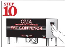
Turn on dishmachine by pressing the "POWER ON/OFF"switch to the "ON"position. Dishmachine will fill automatically and will also activate heater.
