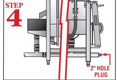
Connect drain at either end of the horizontal drain pipe from wash tank or scrap trap drain.
