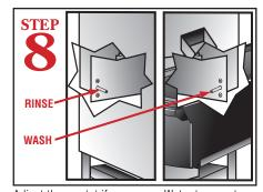
Adjust thermostat if necessary. Water temperature should be 140F rinse and 140F wash for EST44L. The EST44H should read 180F rinse 155F wash.
