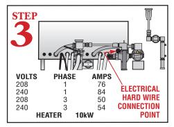
**3 Phase:** Connect the wire with the highest voltage (stinger lead) to L2 on the contactor. L1, L2 and L3 must comply with all local and state electrical codes for sizing of wire and circuit breaker protection. Additional information can be found in the Installation and Operation manual supplied with machine.
