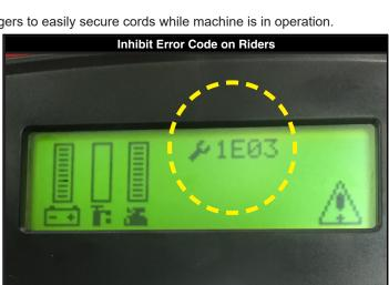
Riders with an Onboard Delta Q Charger do not feature a new light, but instead trigger an inhibit error code on the LCD when operator is charging unit and trying to drive.
