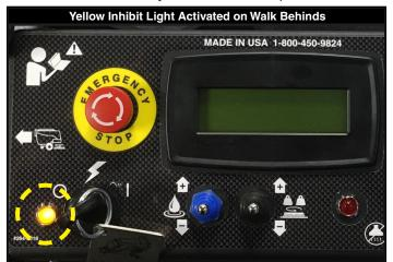
Walk Behinds with an Onboard Delta Q Charger feature an internal inhibit switch and a new light on the dashboard of the CC to illuminate when the equipment won't move due to charging.
