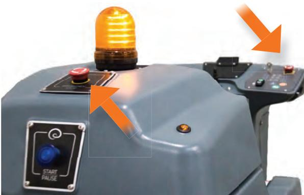
The Brain-enabled scrubber is equipped with two emergency stop buttons
