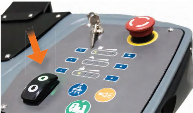
Controls direction machine travels when accelerator pedal is pressed. Pressing upward arrow instructs machine to drive forward. Pressing downward arrow puts machine in reverse mode.
