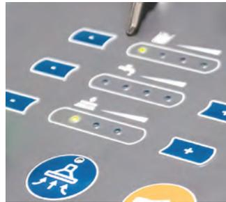
5. If manual cleaning is to be conducted, select desired cleaning settings using the scrubber depth indicator, detergent level indicator and water level indicator adjustment buttons.
