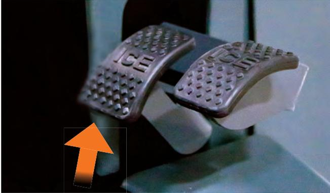
The machine is also equipped with a brake pedal that can be used to control the machine if quicker stopping is needed or when operating on an incline.
