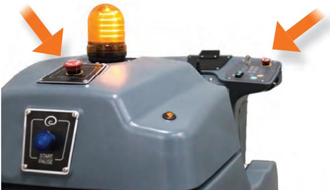
**WARNING:** Only use the emergency stop during an actual emergency, as this function potentially allows fluids in the machine to release onto the floor. To pause operation during autonomous mode, use the rear blue autonomy button.
