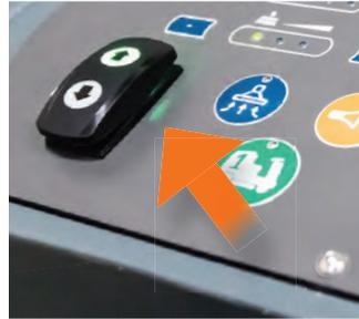
3. The machine is able to operate in forward or reverse. Use directional switch to select desired direction.
