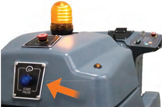
Initiates autonomous (robotic) mode, pauses autonomous mode and resumes operations after a pause.
