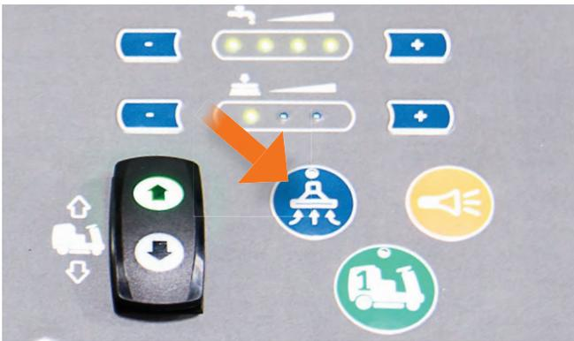
Next, press the vacuum button to turn off the vacuum.
