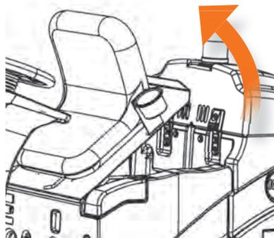
2. Remove the operator seat and the battery box from the scrubber.
