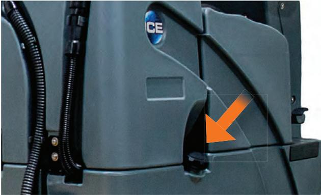
The Brain-enabled scrubber is equipped with a hose to fill clean water port (Machine Components #2) at the side of the machine, and a bucket fill-port located under recovery tank.
