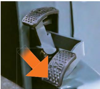
4. To begin driving, press propel (accelerator) pedal. Speed can be adjusted by the force applied to the pedal - light is slow, heavy is fast, before driving the Brain-enabled scrubber
