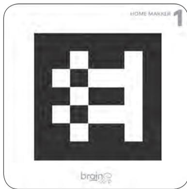
Home location codes should be displayed on a wall, in a well lit location, where there are no shadows obstructing the code. Affix the home location codes to the wall, use a pin, hook or tape to keep it in place. The entire home location code should be clearly visible, not hidden behind furniture or shelving.
