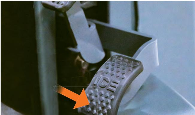
Press propel (accelerator) pedal to drive the machine. Removing pressure from the pedal stops travel. The park brake engages after short delay.
