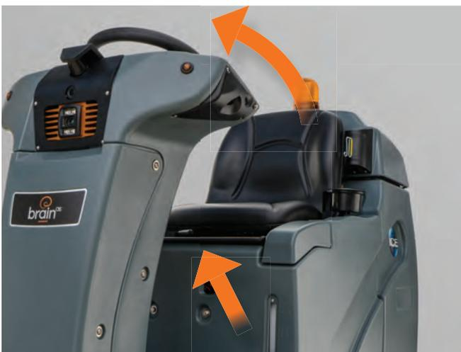
The seat is moved forward and backward using the black lever protruding from underneath seat base. This seat can also be lifted to access the Brain-enabled scrubber battery and brake release instructions and tool.
