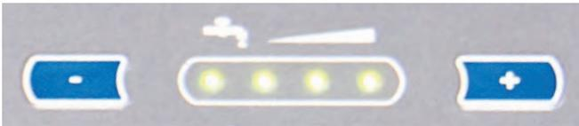
Press the blue plus and minus buttons on either end of the indicator to increase or decrease the amount of water released. The machine allows between 0%-5% of water release.
