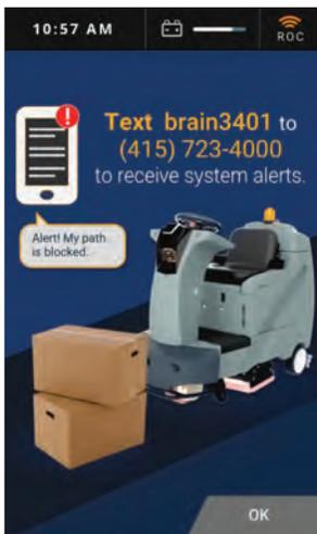
The ROC Indicator is located on the user interface LCD screen in the status bar. When the ROC Indicator is illuminated orange, the Brain-enabled scrubber is successfully connected to the ROC.
