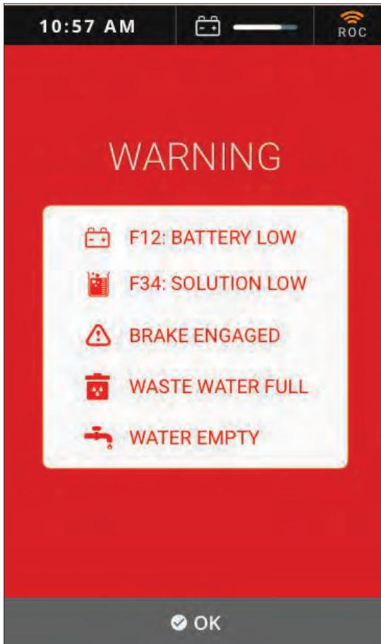
When a fault occurs, discontinue operating the machine until the fault is eliminated. Turn off the machine and resolve the fault. The fault code will be eliminated when the machine is restarted.
