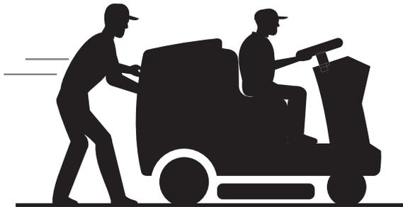
3. Push the machine into a safe location where it can remain until a service technician arrives to perform repairs.
