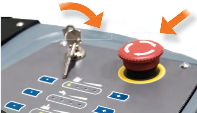
Pushing this button in an emergency shuts off all manual functions. To restart machine, reset the emergency stop button, turn off the momentary key/ignition switch and then turn on the key switch.
