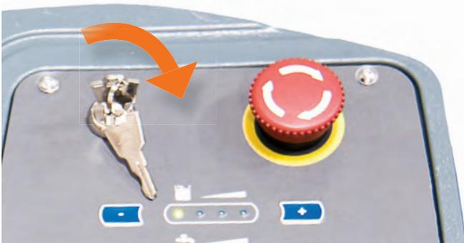
Insert momentary key into ignition and turn clockwise to start power.
