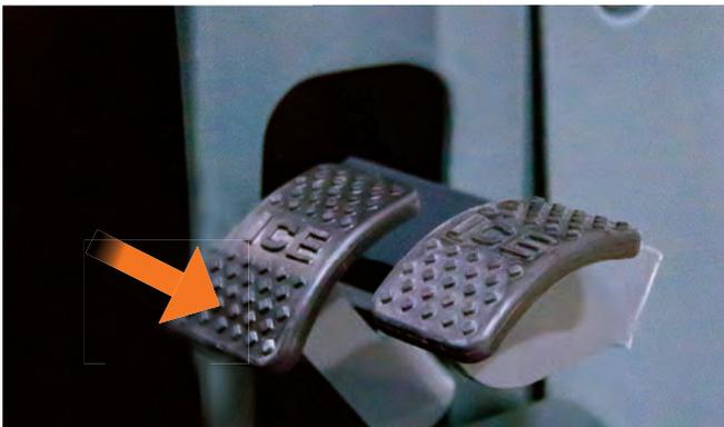
Removing pressure from propel (accelerator) pedal stops travel. The park brake engages after a short delay.
