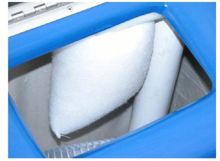
example of vacuum filter bag in the recovery tank
