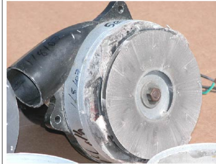
serious damage to vacuum motor cause by not using vacuum filter bag in the recovery tank
