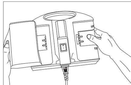
Turn on the Battery Charger by pressing the switch; the switch should light up to indicate the power is on, and the battery packs are now charging, which is indicated with an LED (red – charging/green – fully charged or no batteries inserted) and voltage. It takes approximately 5 hours to fully charge an empty set of battery packs.
