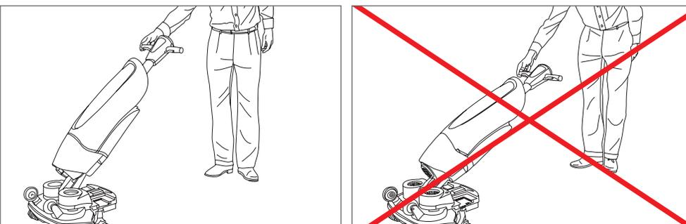
The i-mop scrub deck is designed to get as close as possible to walls. Approach walls diagonally with the edge of the i-mop and continue along the wall.
