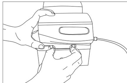
When the battery packs are charged, press the plastic tabs (blue or grey) on the battery packs together and slide them out of the charging dock.
