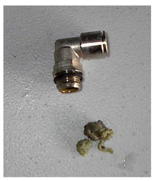
Inspect and clean out any blockage. 95% of the time a no flow or no foam issue can be traced back to a blockage in the tank right angle connector.
