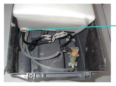
Remove the right angle connector from the tank.
