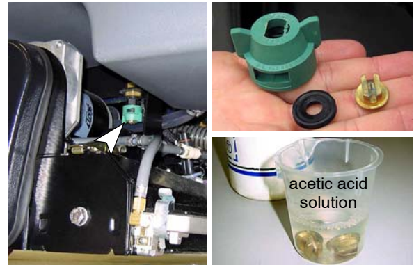
ReadySpace Spray Nozzle GREEN CAP / TIP #11002 p/n 575283000
