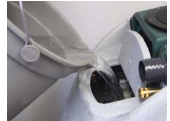
Pour 2 or 3 gallons of clean water into Solution Tank
