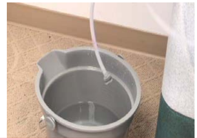
Place Chemical Feed Hose into Rinse Solution
