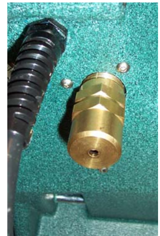
Replace Spring and thread Brass Knob back onto regulator body
