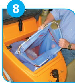
Remove and clean the solution tank (blue bag) and allow to air dry; then clean the recovery tank.
