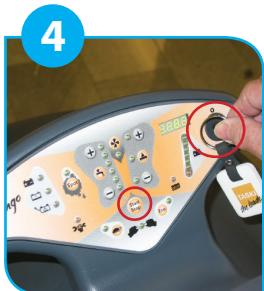
Turn machine on and hit 'start' button to begin cleaning.
