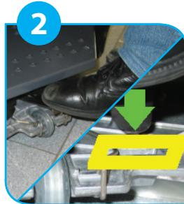
Mount squeegee with 'click' mechanism and attach the suction hoses.
