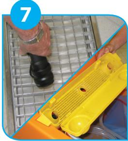
Drain recovery tank with the draining hose. Remove and clean the yellow debris tray.
