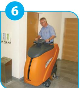
Clean the required floor area. Afterwards switch off cleaning functions with 'stop' button.
