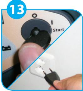
Move unit to charging location, turn unit off and plug into the battery charger.
