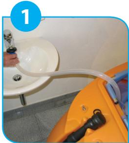
Fill solution tank (blue bag) with properly diluted chemical.
