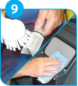
Clean the fresh water filter and the vacuum motor filter.
