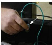
Feed the green wire thru hole on the back of the handle panel.
