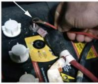
Remove the red battery charger wire from the positive battery post.
