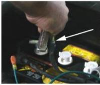
Using a 1/2 in socket wrench, remove the nut holding the negative battery cable.
