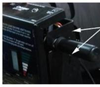
3. Using a Phillips screwdriver, loosen the 5 screws on the handle panel. 1 screw is on the back of panel and 2 screws are on each side of the panel.
