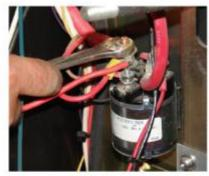
25. Loosen the nut holding the red wire to the "hot" side of the solenoid with a 1/2 in wrench.
