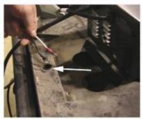
17. Feed the battery charger wires (white and black wires) thru the hole on the cover.
