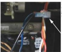
Attach the wire connector end of jumper wire to the switch.
