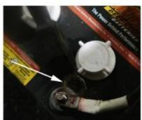
Remove the black and white battery charger wire from the negative battery post.
