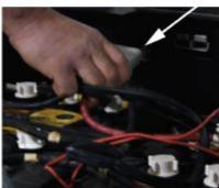
Disconnect the batteries by pulling the gray charger plug apart.
