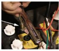
Using a 1/2 in socket wrench, remove the nut holding the positive battery cable.
