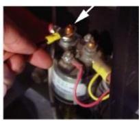
26. Attach the ring end of jumper wire to the "hot side" of solenoid and tighten nut.
