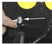
12. Using a 7/16 wrench, remove the nutted bolt (on the underside of the cover) which holds the old battery charger. Set the bolt aside to use on the new battery harger.
