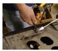
Pull the battery charger wires thru the cover.
