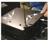
16. Using a Phillips screwdriver, install the 2 brackets (included with the new battery charger) onto the battery charger.
