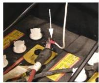
19. Using a 7/16 in socket wrench, attach the white wire from the battery charger to the positive battery cable and tighten cable.
