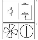
Allow the suction unit to continue running until the rest of the dirty water has been sucked into the hose.
