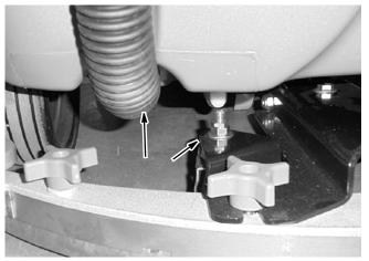
When squeegee assembly strikes a wall with excessive force, the left side of the squeegee lift bracket will crush drain hose.
