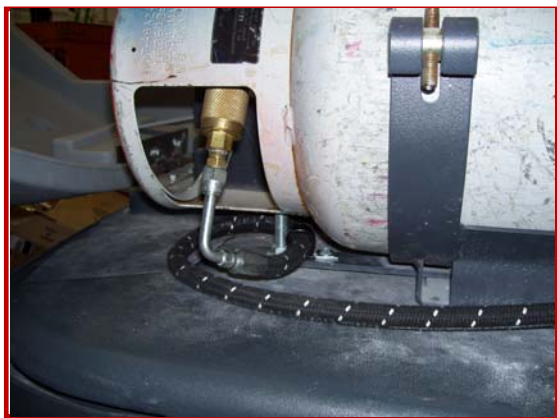
Old Hose Routing with potential for hose to overlap and press on the fitting causing leak
