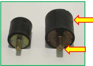
EDGE uses large and durable Isolators, which do the hard work on the machine. They are 1" diameter with 5/16" stud bolts. Shown next to alternative that is smaller in both areas. Many alternative isolators are also softer, which is required due to less powerful motors. Smaller/Softer isolators typically require more frequent replacement and can fail from impacts.
