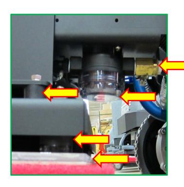
Oversized Solution Filter (stainless screen) and Brass gate valve for easy access and service.
