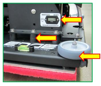
EDGE decks comes with a hour meter to track isolator time, for scheduled replacement every 250 hours. An affordable kit includes new isolators, bolts, and a hour meter.
