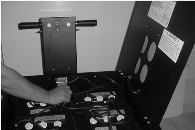
When the machine is shipped with batteries, the machine will arrive with the battery pack disconnected from the machine.
