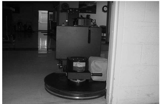
**NSS** recommends transporting the machine to the work site with the front of the machine in the operating position and the brush switch in the off position. This will reduce the potential of damage to the Flexiwall Shield and Pad Driver when moving through stock/storage rooms and double swinging doors.
