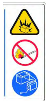
WARNING LABEL - Batteries emit hydrogen gas. Explosion or fire can result. Keep sparks and open flame away when charging. Located on bottom side of recovery tank.
