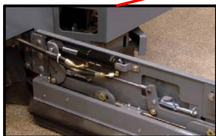
Right Side Squeegee Lift Cylinder
