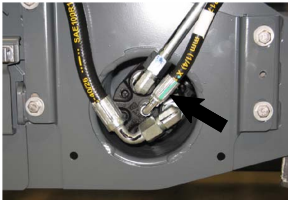
Install additional fitting on to front brush motor
