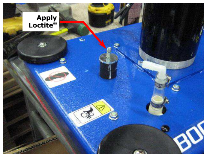
Figure 18 – Applying Loctite® to Upper Isolator Threads
