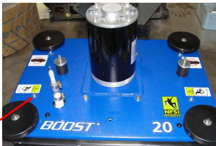
Figure 16 – Attaching Nuts to Lower Isolator Studs
