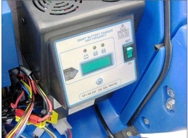
Figure 7 – WET/GEL Switch Set to GEL
