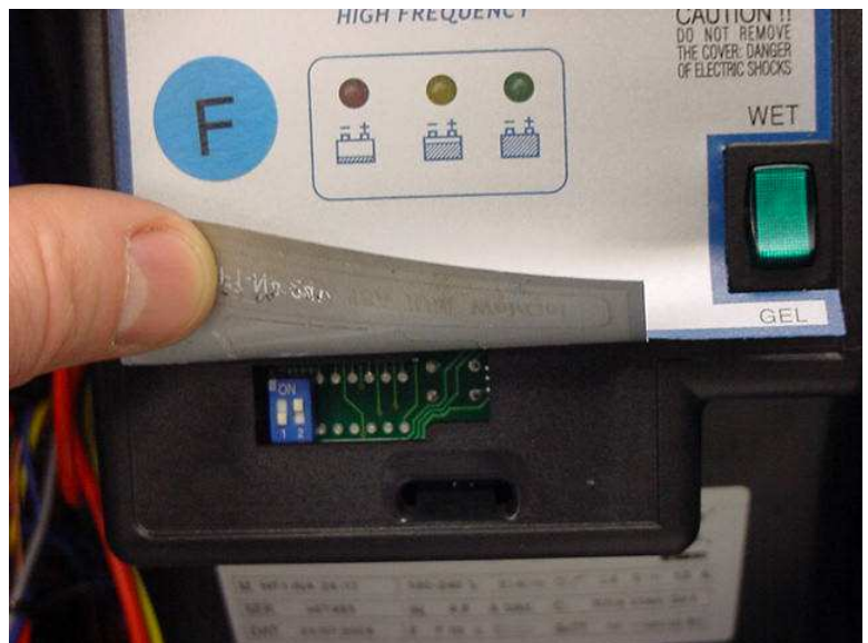
Figure 6b – DIP Switches on Current Style Chargers
