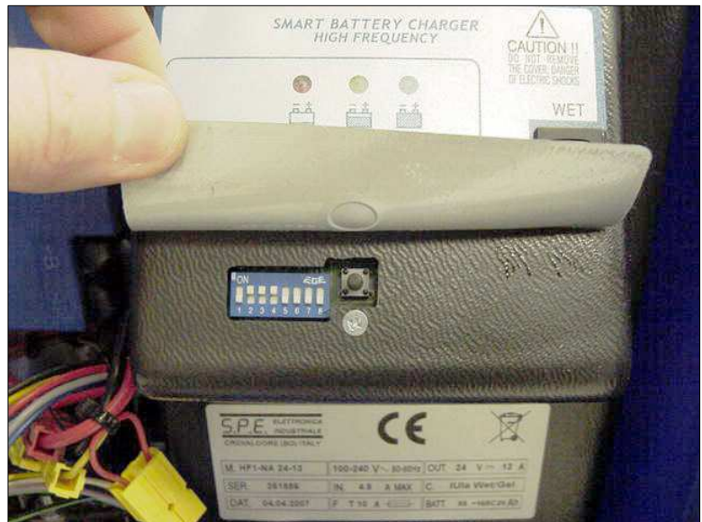
Figure 6a – DIP Switches on Old Style Chargers
