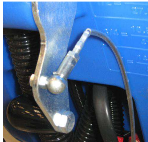
Figure 2 – Cable Positioned Incorrectly
