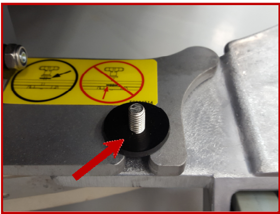
Insert Nylon Washer Above Support Bracket
