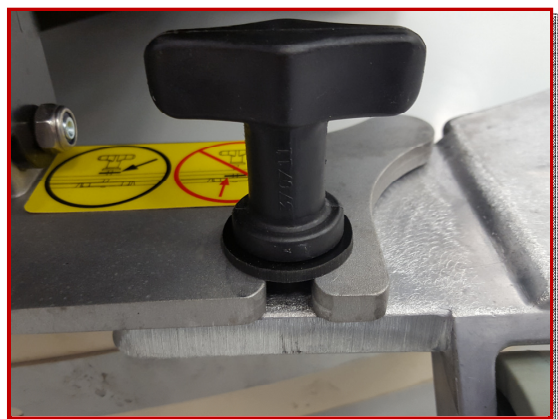
Thumb Nut Installed **DO NOT USE ANY TOOLS TO TIGHTEN**
