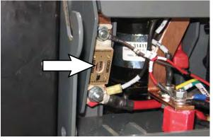
If your machine is not running autonomously check the autonomy On/Off switch. It is located by the hour meter. Always check to make sure it is turned on. 1 is on 0 is off.
