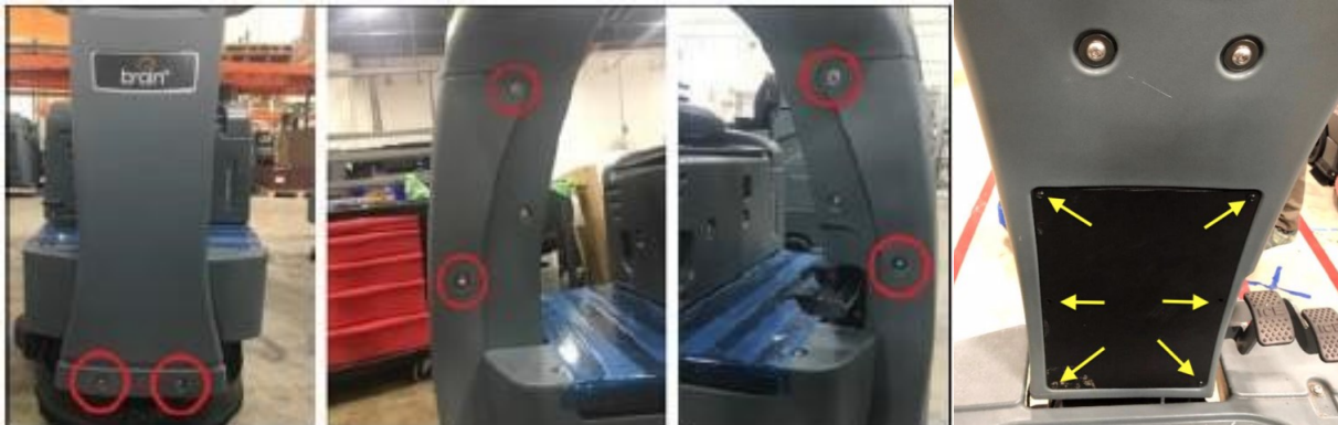
Removing both access panels
