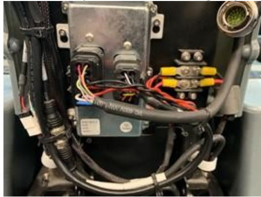
Example of a Bad Steering amp (Damaged wiring)
