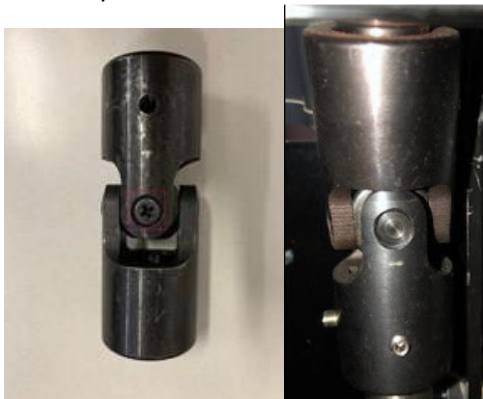
Example of a U-joint in good condition
