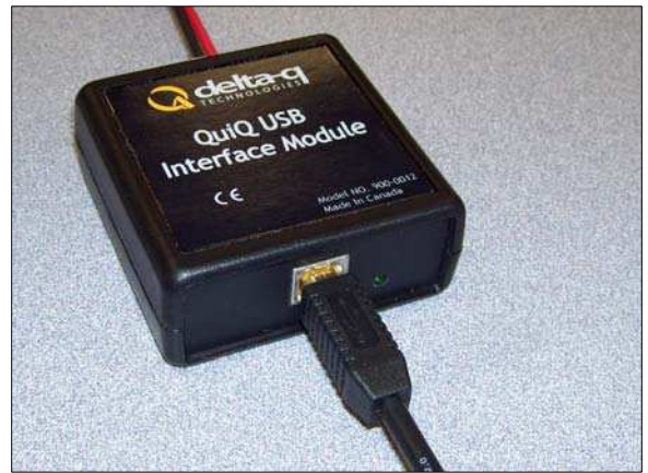
Figure 4 – Connect “B-type” USB Plug to USB Interface Module
