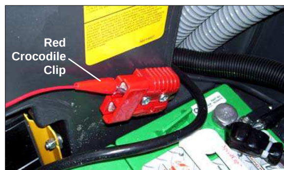
Figure 2 – Attach Red Crocodile Clip to Positive Side of Battery Pack Connector
