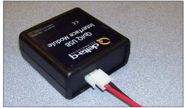
Figure 3 – Connect Two-conductor Plug to USB Interface Module
