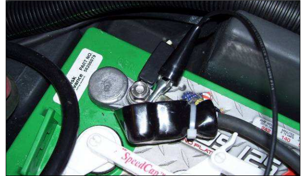
Figure 1 – Attach black alligator clip to negative battery terminal
