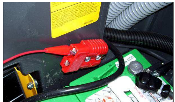
Figure 2 – Attach red alligator clip to positive side of battery pack connector
