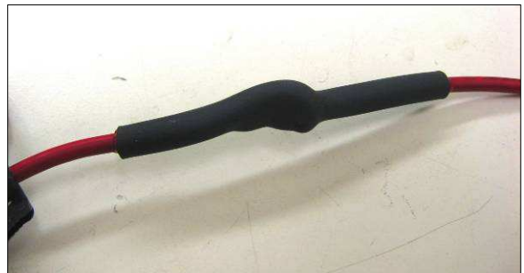
Figure 6 – Heat-shrink Insulation Over Splice
