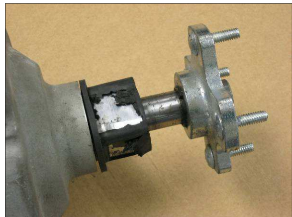
Figure 2 - Damaged Neoprene Mounting Sleeve
