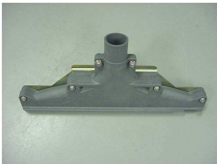
Fig 6- Install new vac shoe bracket, reinstall mounting hardware and torque to 67 in-lbs.
