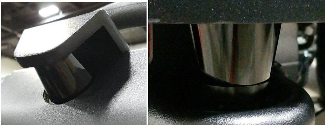
Brain / ICE RS26 Slanted (upper) and Planar (lower) LIDARs
