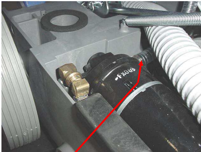
Fig 4- Design change to improve pump priming resulted in pump being re-orientated such that inlet & outlet ports are on the LH & RH side vs top and bottom. Refer to pump bypass kit 56265226 or 56265227.
