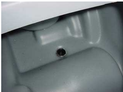
Barb is pressed into fitting in solution tank
