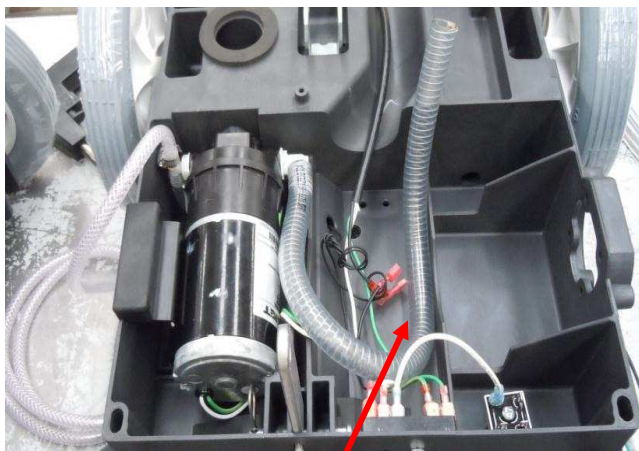
Fig 4 - Incorrect Hose Routing
