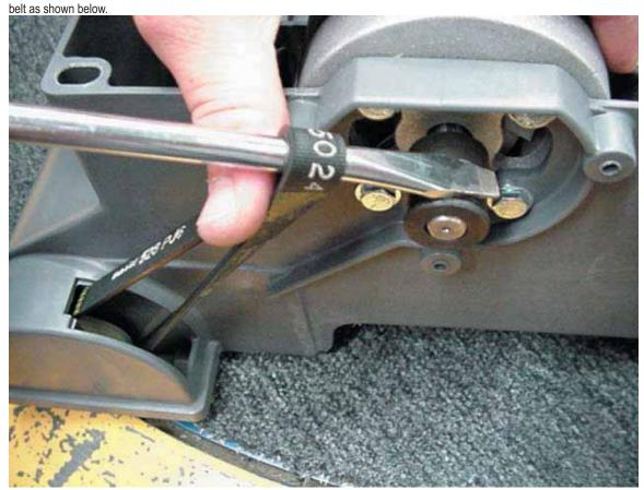
**Step 3:** While maintaining pressure with your thumb, slowly begin rotating screwdriver about the sheave as shown below.
