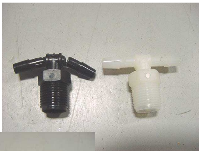
Fig 3- New Tee fitting is made from Nylon, has 2X the tensile strength of the original fitting made from HDPE and is significantly more ductile to prevent fractures.
