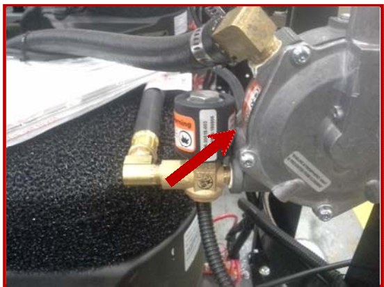
Prior to addition of Brass Spacer (PN 56383971). Notice Interference fit.
