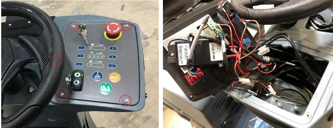
Disconnect the BCM fan power connector
