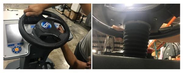
Use a 7/8 socket wrench to remove the nylon nut and washer that secures the steering wheel. Wiggle the steering wheel back and forth and pull up to remove. Once freed, realign and reassemble.
