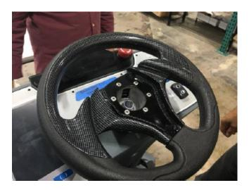
Reconnect the red battery coupling. Turn the key to power on the unit to ensure proper start up and system operation.
