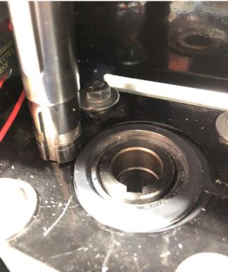
The Steering Encoder can now be slid off from the bottom of the steering shaft and replaced with a new one.
