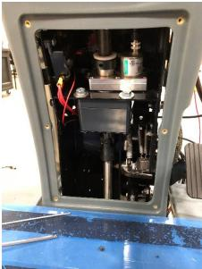
Spin the wheel to provide access to these two set screws.
