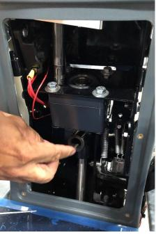
Push the steering wheel down to move the shaft into place. It should move through the drive motor and lock into the U joint below. Make sure the keys all line up and the wheel is pushed all the way down before re-securing the four set screws. Raise the collar back up and tighten the hex screws.
