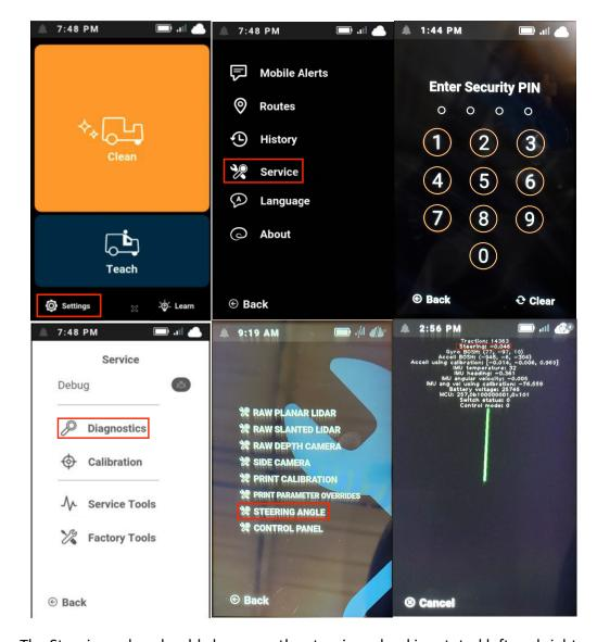
The Steering value should change as the steering wheel is rotated left and right.
