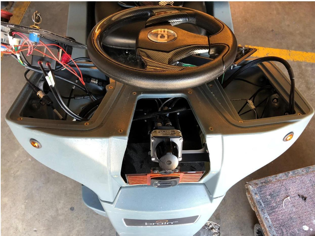
To mount the Antennae, loosen/remove the Slanted LIDAR hex screws. It is **VERY** important to be careful with this sensor. Do not disconnect the rear cables, but rather keep them tethered to allow the Slanted LIDAR to be maneuvered so the antenna bracket can be mounted. Be **VERY careful** not to scratch or damage the LIDAR.
