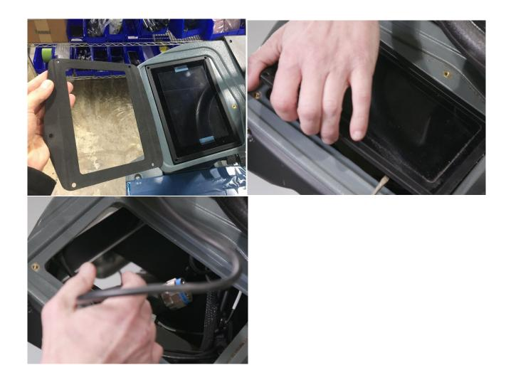
Install the new touchscreen and feed the cable back through the steering column. Reconnect the touchscreen trunk to the BCM, Reconnect the red battery coupling and power on the unit.
