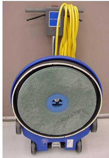
Fig 1-Place your machine in the handle-up storage position to gain access to pad and pad holder.
