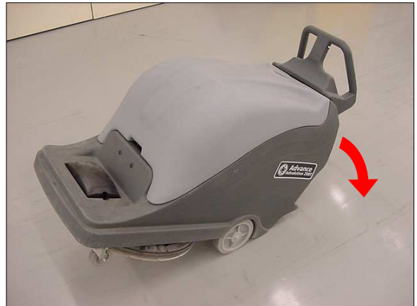
Figure 2 – Tipping Machine to Access the Pad Tilt Adjustment Hardware
