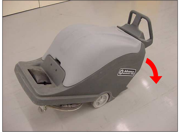
Figure 10 – Tipping Machine to Access the Front Housing Mounting Bolts
