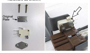
3. Mount the bracket assembly to machine with hardware as shown.
