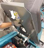
12. Reinstall fuse into telemetry harness.
