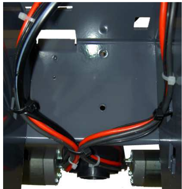
Fixation of the cables on the chassis (from the side of the electronics)
